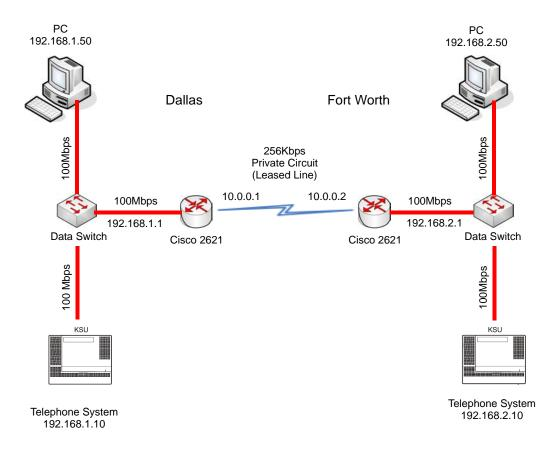
Figure 6-8 Common Network with Cisco Router
