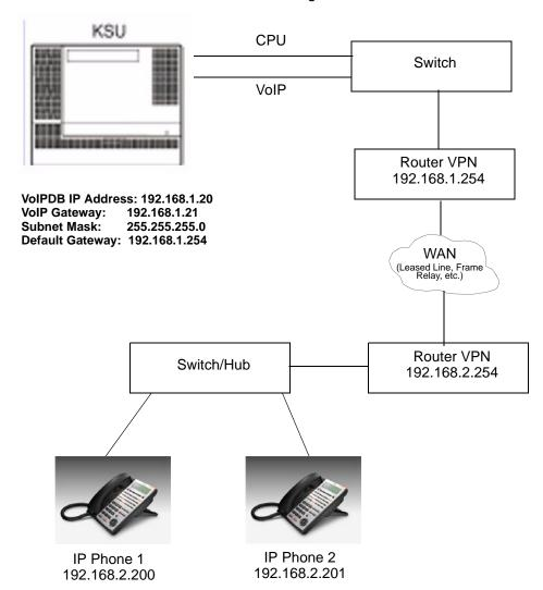
Figure 9-5 Example Configuration 3 - Static IP Addressing, Routed WAN
