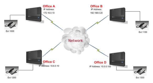
Figure 3-1 Example of SL1100 IP Network Configuration
