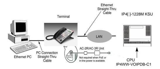
Figure 9-2 Typical Network IP Connection
