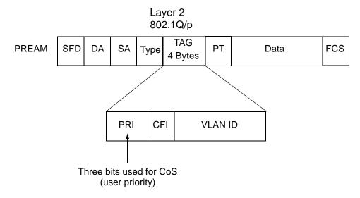
Figure 6-1 Layer 2 Diagram (802.1Q)
