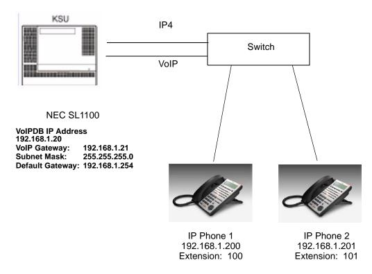
Figure 9-3 Example Configuration 1 - Static IP Addressing, One LAN
