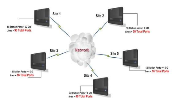
Figure 13-1 System Capacity Diagram
