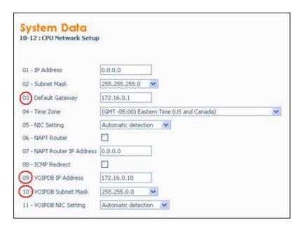
Figure 9-26 System Data 10-12: CD CP00 Network Setup
