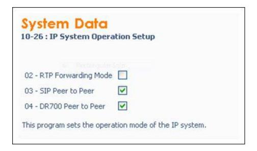
Figure 9-25 IP System Operation Setup
