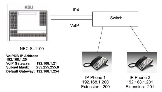
Figure 9-4 Example Configuration 2 - Dynamic IP Addressing, One LAN
