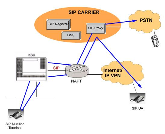
Figure 7-1 Common IP Network using NEC SL1100 SIP Trunk
