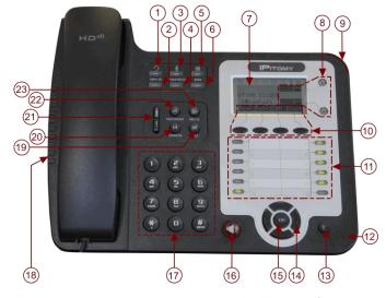
Figure 4 IPitomy IP320 Buttons and Hardware Definitions
